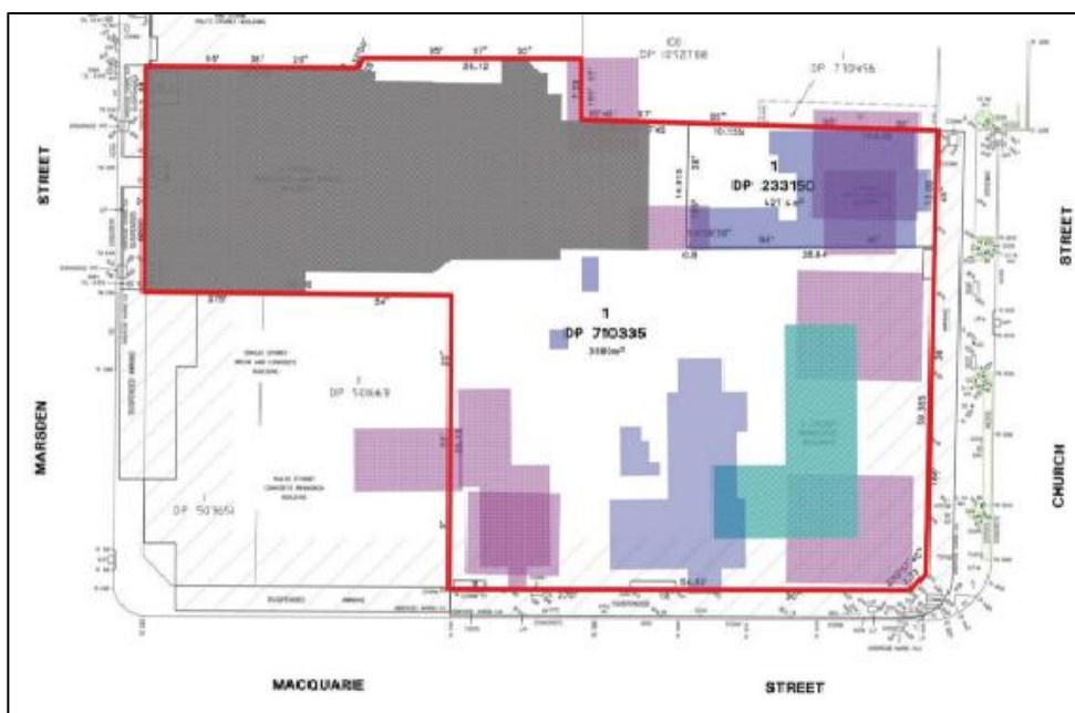
Figure 31. Likely significance patterns on the subject site as assessed in GML report. Key: Blue: national. Violet: state. Indigo: local. Grey: none. 43
